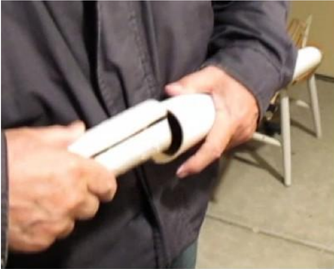
Figure III-10: Sliding the longitudinally cut segment of tubing in the front segment of the telescope tube.
