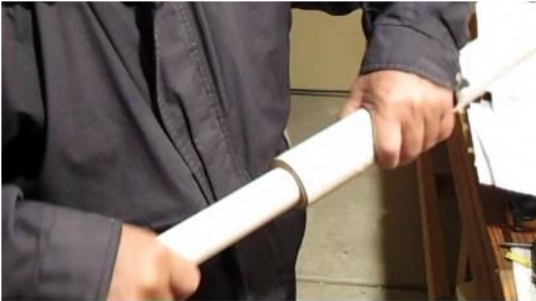
Figure III-8: Inserting the drawtube into the back of the telescope tube.
