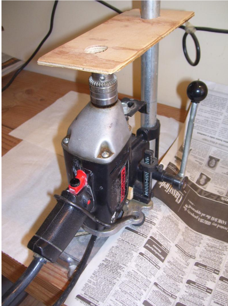
Figure II-2: The variable speed drill (mounted upside down), its mount and the platform that together are used to do the optical work on the telescope lenses.
