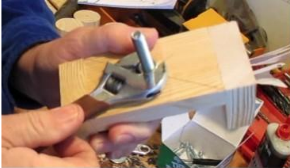
Figure IV-18: Mounting of the two 5/16-inch stove bolts in the two sides of the saddle.
