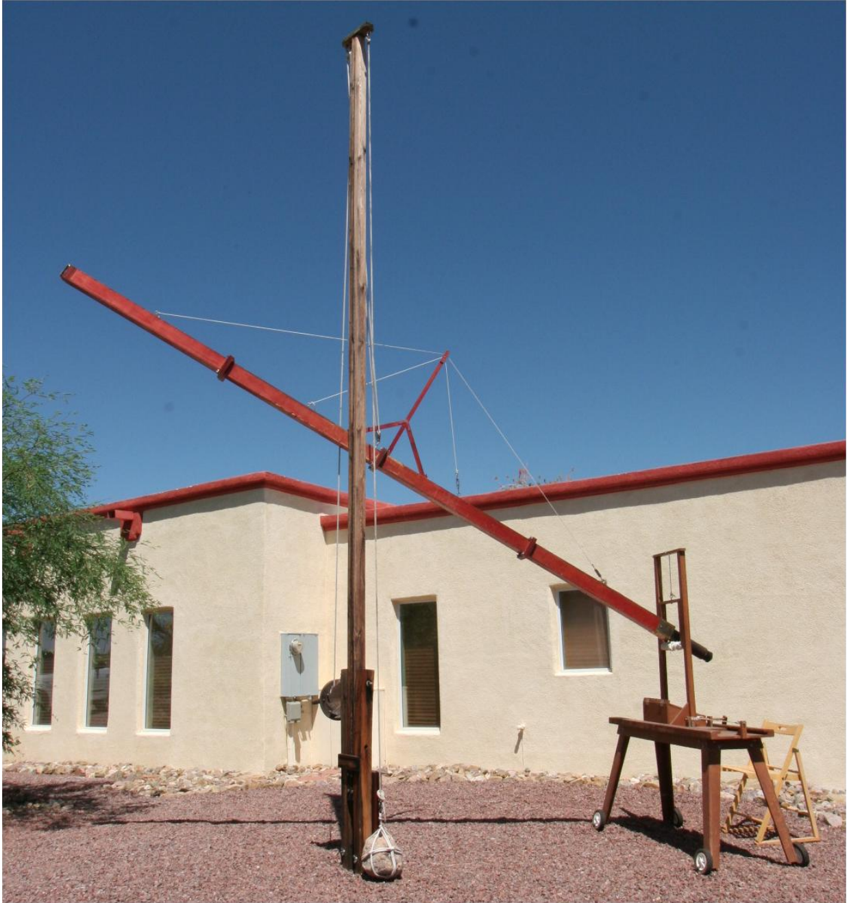
Figure I-3: AB's 17-foot replica of the long-focal, non-achromatic refractors and mounts of the second half of the 17 th century.
