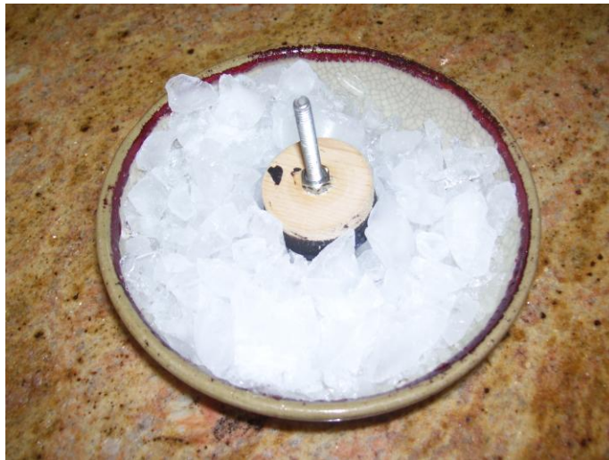
Figure II-10: Removing the lens from the spindle is made simple by setting the lens/spindle in a bowl of crushed ice for several minutes.
