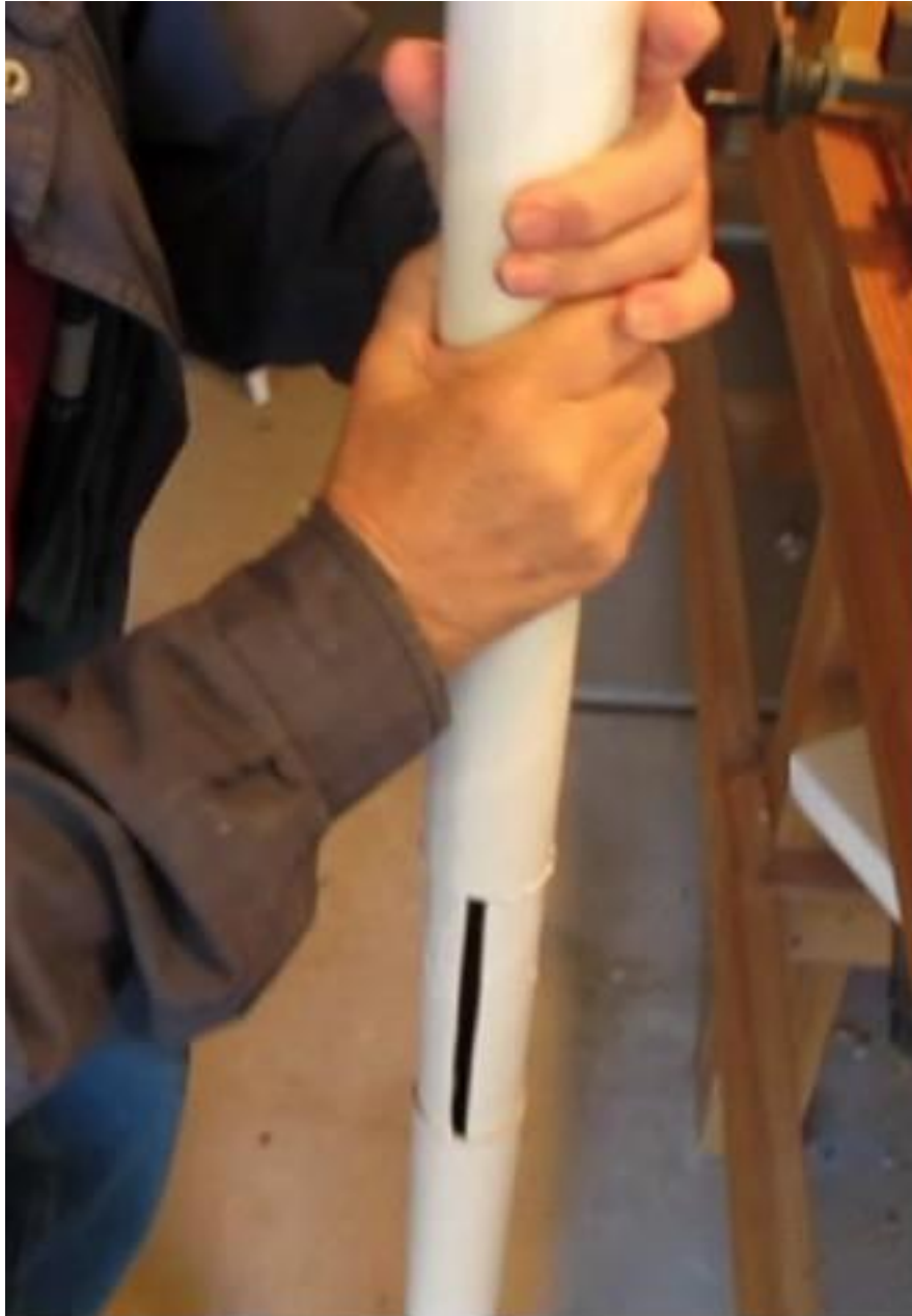
Figure III-11: Joining the back segment of the telescope tube to the front segment of the telescope tube.
