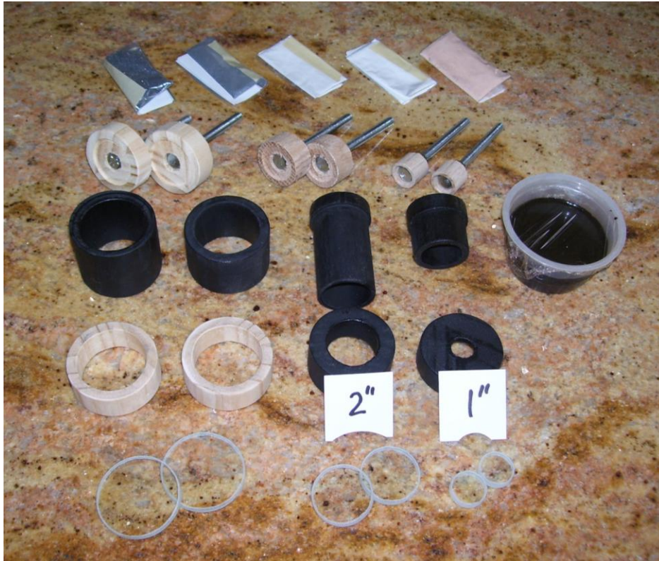
Figure I-11: The kit supplied by Ken Press needed to grind and polish the single element objective lens and the two Keplerian eyepiece lenses described in this manual. From left to right in each row:
