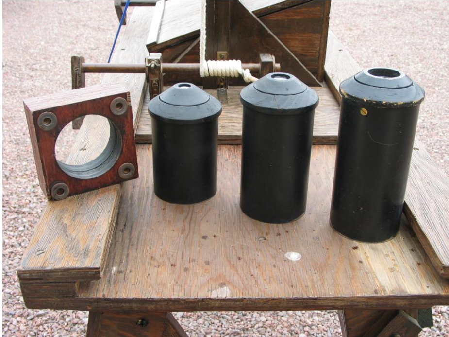
Figure 1-4: The single element, 2.8-inch clear aperture objective lens and the three Huygens eyepieces (50x, 100x and 150x) of AB's 17-foot replica telescope.
