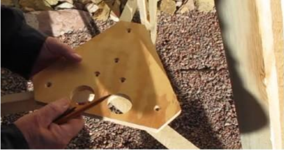
Figure IV-13: Photo showing how to prepare for gluing and drilling the pilot holes in the three shelf supports.
