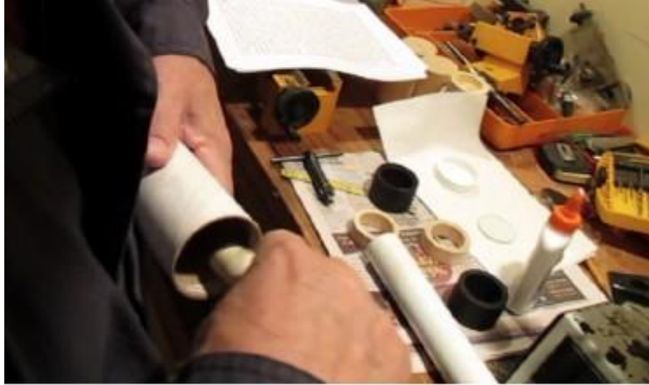
Figure III-2: Swabbing Elmer's glue in the front end of the outer-tube section of telescope tube.
