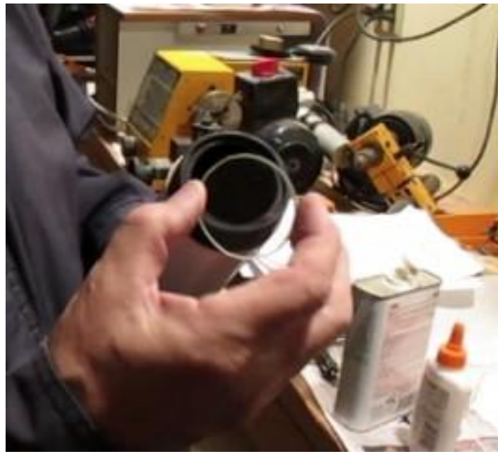
Figure III-4: Inserting the objective lens, with its convex side up, into the retaining ring of the objective cell.
