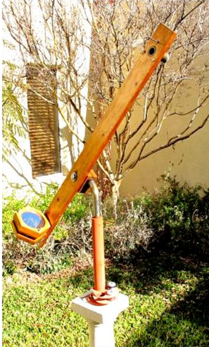
Figure I-1: A simple, 4-inch, 36-inch focal length (FL), Newtonian Reflector with a simple equatorial mount on a cement pillar in the atrium of AB's house. This telescope also has a tripod that AB uses when he is camping or wants to observe at a different location. Building this kind of telescope and mount requires only simple wood and metal working tools.
