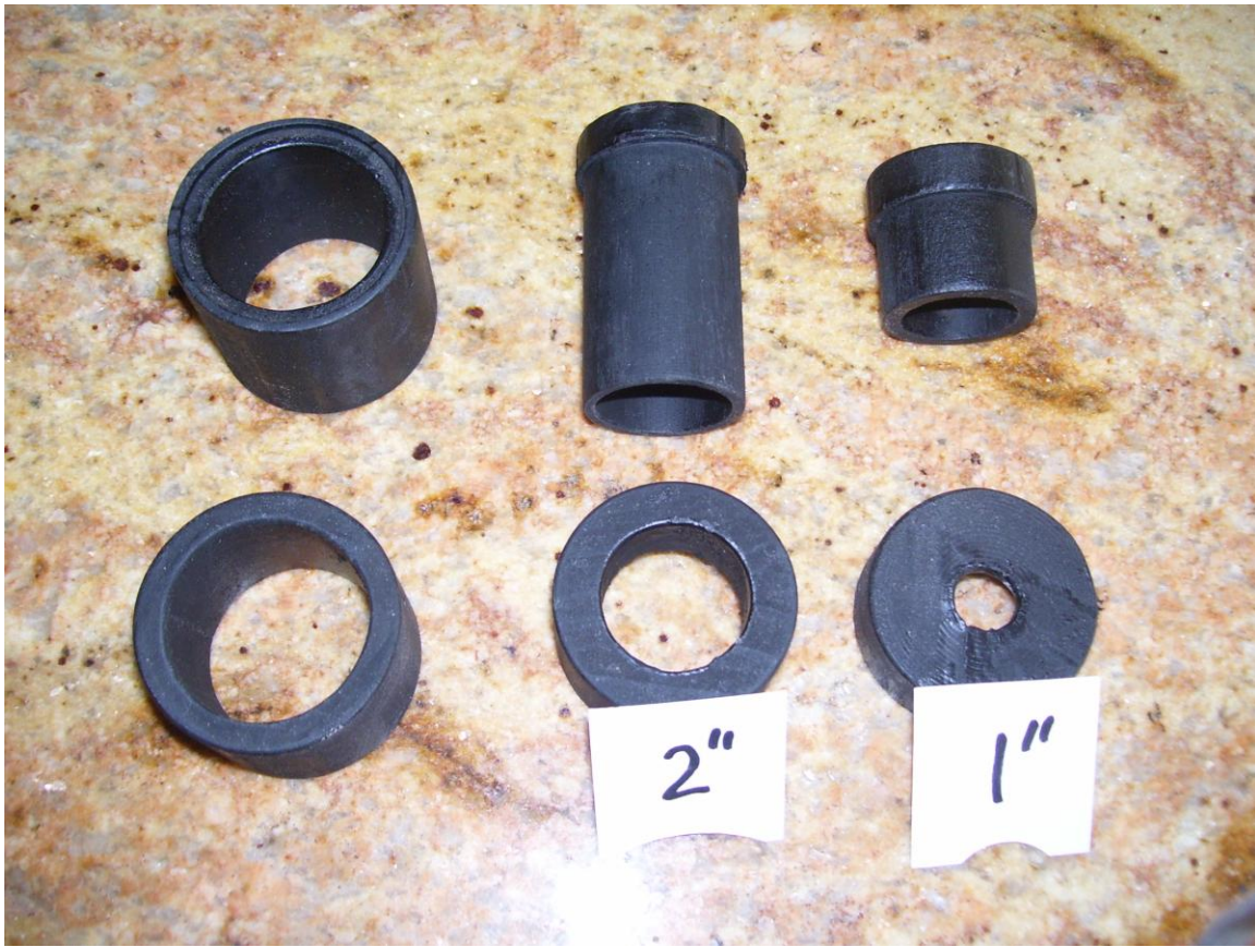
Figure II-1: The two components of the objective lens cell and those of the two eyepieces that have been spray painted with flat black paint.
