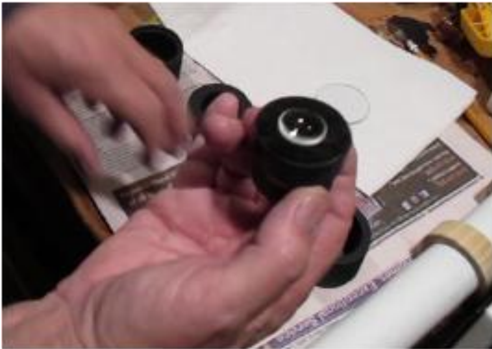
Figure III-1: Mounting an eyepiece lens in its barrel.
