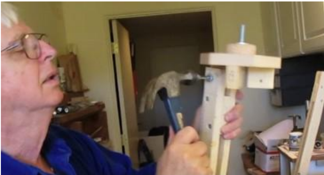
Figure IV-10: Photo of joining the legs to the tripod support structure.
