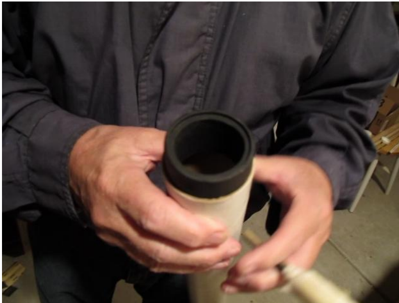
Figure III-3: The correct position of the back segment of the objective cell in the front end of the telescope tube, with the \frac{1}{8} -inch tall, 1\frac{3}{4} -inch ID retaining ring visible.
