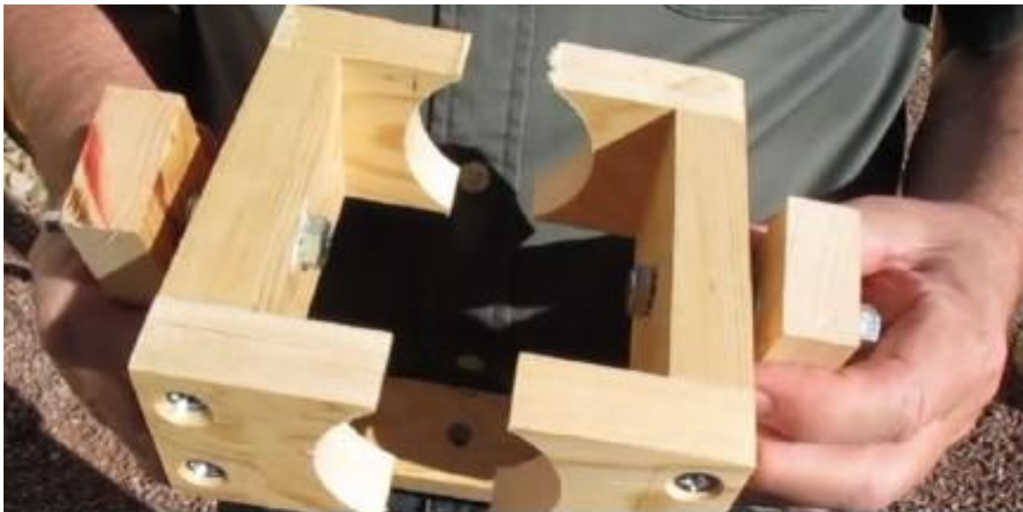
Figure IV-19: Photo of the finished saddle parts mounted in the yoke.
