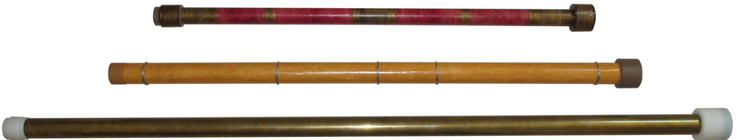
Figure I-5: Replicas of three of Galileo's telescopes made by the authors.
