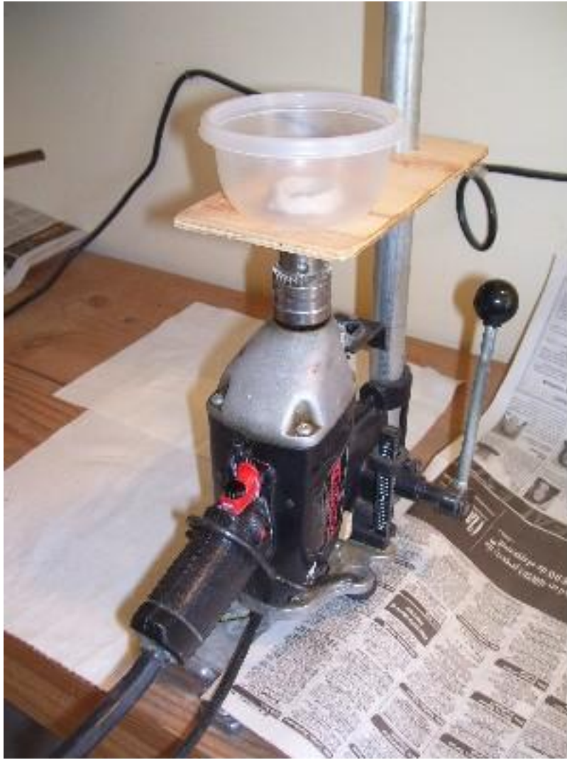
Figure II-5: The placement of the catch tub on the drill platform.
