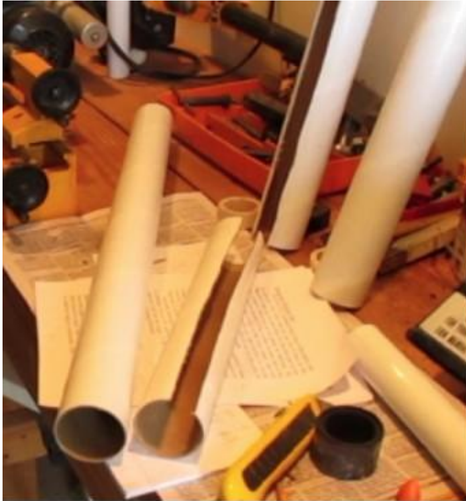
Figure III-9: The segments of tubing after a strip, \frac{3}{4} of an inch wide, has been cut from them.
