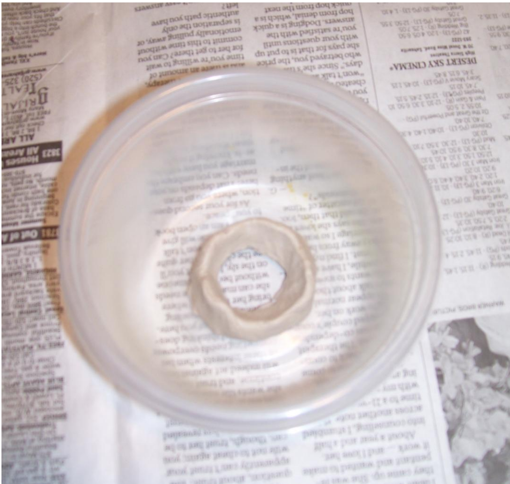
Figure II-4: The plastic “catch tub” used to catch grinding grit, mud, polishing CeO and water from dropping onto the inverted drill.
