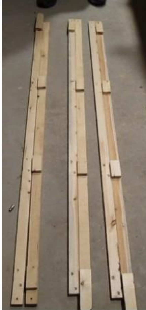
Figure IV-9: Photo of how the three pairs of long leg boards should look after drilling (and countersinking) the hole in the boards.
