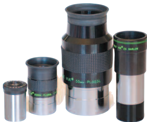
The eyepiece on the far left has a barrel diameter of 0.965 inches. The 20mm Plössl eyepiece to its right has the standard barrel diameter of 1¼ inches. The very large eyepiece in the “center,” a 55mm Plössl, has the largest commercially made barrel diameter of 2 inches. The 2x Barlow lens at the far right accepts eyepieces with 1¼-inch barrel diameters (they are inserted at the top and secured with a thumbscrew (not visible).
