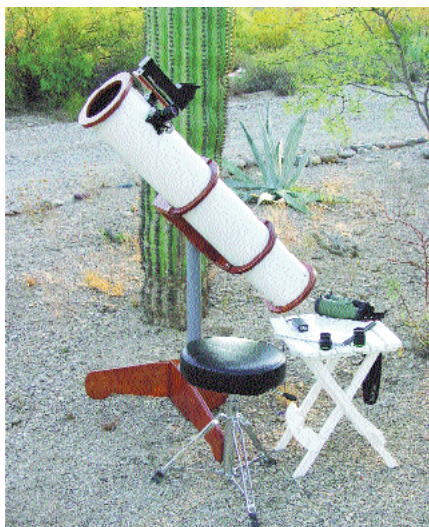
A favorite scope of mine is this 6-inch diameter Newtonian Reflector mounted on a simple altazimuth pipe mount that I made a few years ago. It is quick and easy to set up and fun to use. This is a "manual" scope so I have to move it around by hand.
