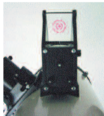
Above. The view through a Telrad, one of the most popular reflex-sight finders. To use, position an eye 6-inches or so behind the slanted glass plate to see the bulls-eye for aiming the scope. These finders are natural and fun to use — kids really like them.
