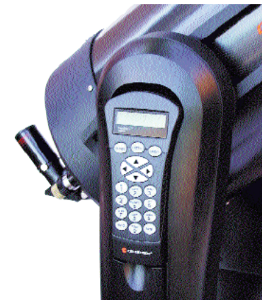
The handcontroller on a SCT telescope with GO TO technology. Databases of objects are accessed through the keypad — similar to phone number lists on cellphones.
