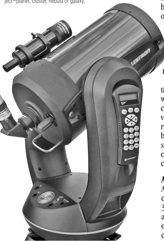
Celestron GOTO SCT showing the hand-controller in an arm of the Alt-Az mount. As with many GOTO mounts, the telescope has to be aligned to two bright stars using prompts from the hand controller before it can find and follow other objects.
