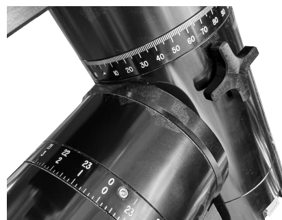
Many equatorial mounts, including cheap ones, incorporate Setting Circles that are scales which could be used to find objects in the sky using the celestial coordinate system of Right Ascension and Declination.
