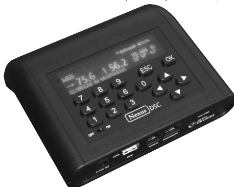
Digital Setting Circles (DSCs) is a display/input box that connects via wires to encoders attached to the telescope's two axes—either Alt-Az or Equatorial. DSCs are meant mainly for manual mounts. After aligning the scope to 2 stars, using prompts from the display, the display will guide you in pushing the scope to any selected object—planet, cluster, nebula or galaxy.
